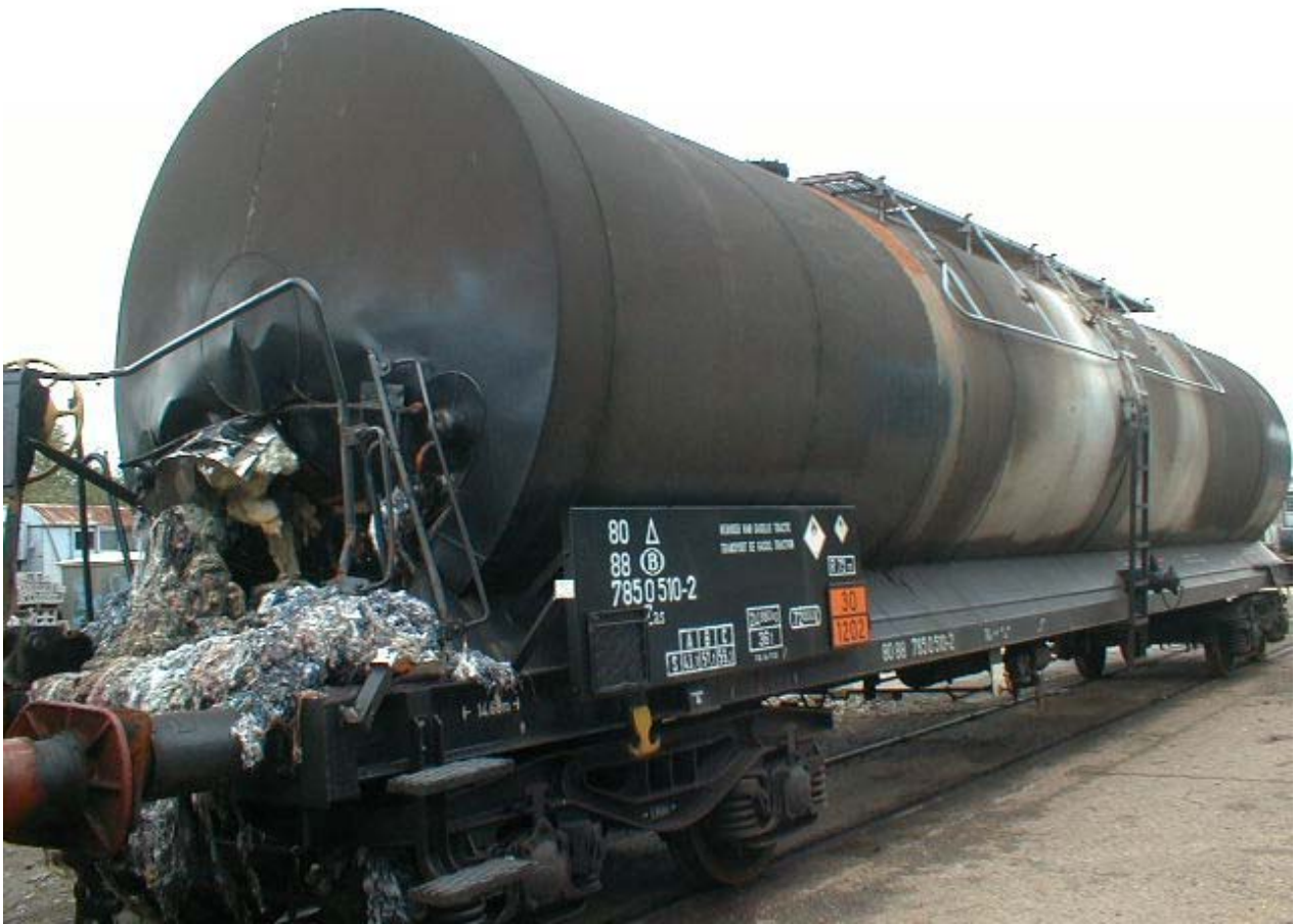
Damage (rupture) to the tank (after clearing work was completed)
