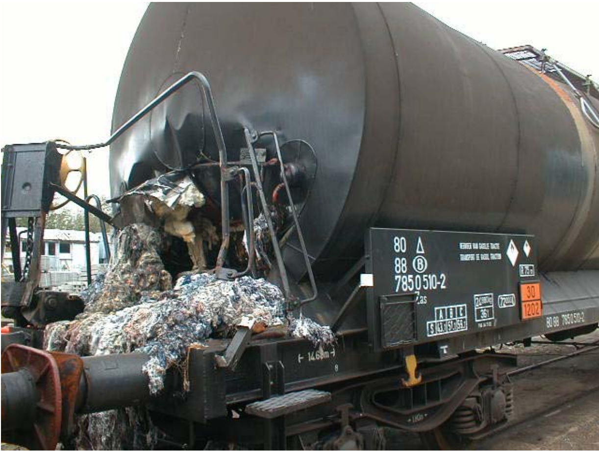
Damage (rupture) to the tank (after clearing work was completed)
