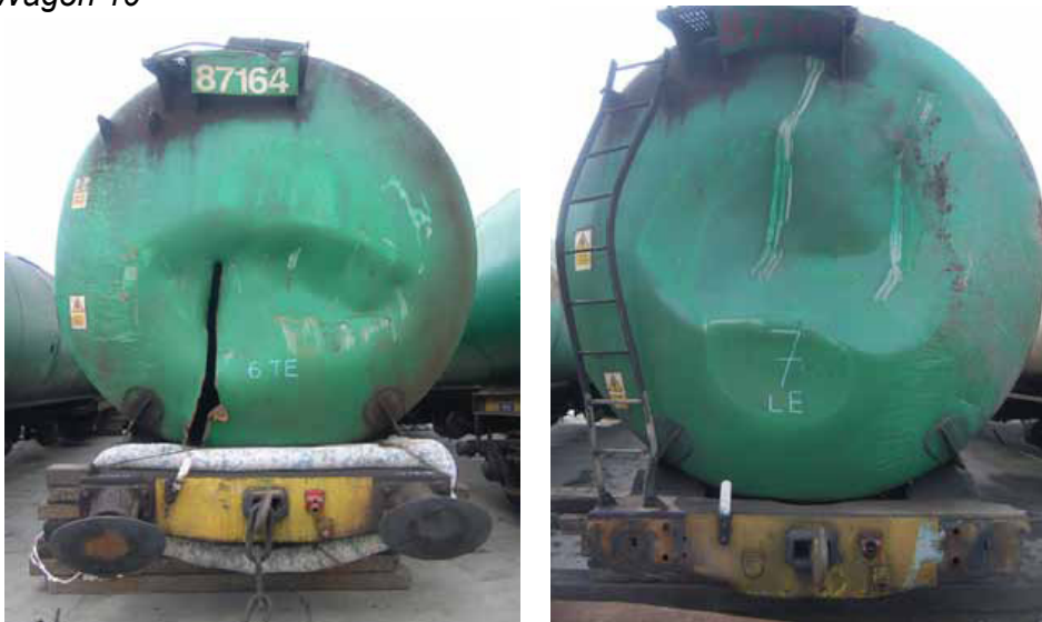
Vertical gash on the tank of wagon 6 (left) caused by the adjacent drawhook on wagon 7 (right)
